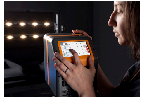
Smart Touch user interface on the ProMetric G2 imaging colorimeter enables quick setup.
