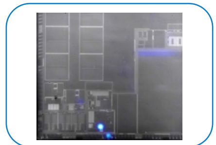
Photoemission on IC using water cooled SWIR InGaAs camera, with 20x objective, exposure time 30s
