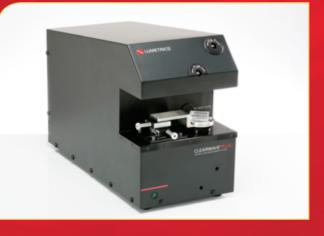
In 2015 Lumetrics was awarded a patent for an apparatus (now known as the ClearWave Plus) that measures the optical performance characteristics and dimensions of an optical element using a Shack-Hartmann wavefront sensor and a low coherence interferometer. This is a major improvement on current contact lens manufacturing inspection methods.
