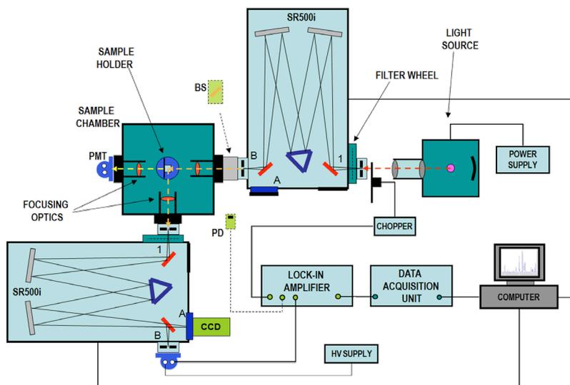
Above: Example of layout for Fluorescence spectrometer
