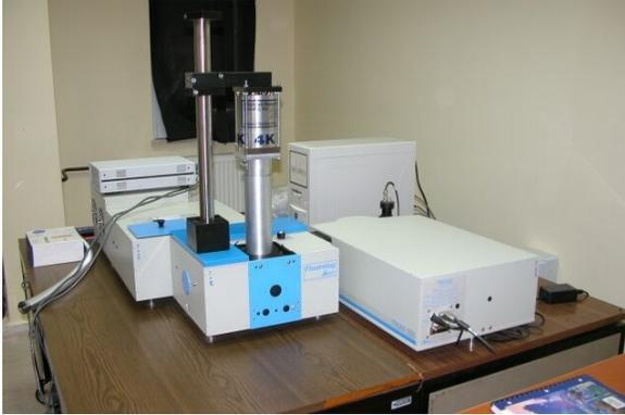
CS202SE-DMX1-AL Installed on Jobyn Yvon Spectrometer.
