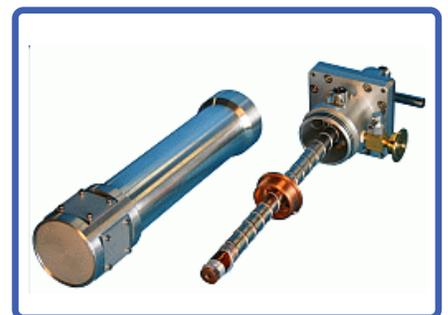
The above picture shows a complete system with the radiation shield mount and vacuum shroud. The transfer line, temperature controller and vacuum pump are not shown.
