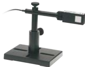
PD300 with filter installed
