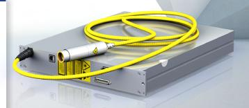
Thulium Continuous Wave (CW) Fiber Laser Modules are available in air-cooled units, 10-50 W or water-cooled modules, 50-200 W. These compact modules can be purchased for single-mode or multi-mode operation with wavelength range of 1900-2050 nm. IPG Thulium modules are attractively priced for OEM's and integrators and serve a wide range of medical, materials processing and laser pumping applications.
