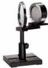
Beam splitter installed – reflected beam on sensor
