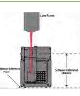
Calibrated beam path for precise focus spot location
