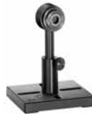
PD300R Filter installed
