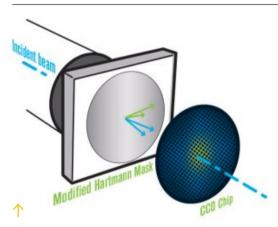
PHASICS® technology was introduced to overcome the Shack-Hartmann sensor limitations, especially resolution. This ultra-high resolution enables accurate wavefront measurement for robust calculations of beam parameters.
