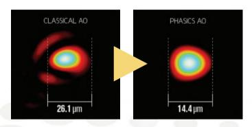
↑ Correction after the last parabola without any additional device to achieve the best possible focal spot
